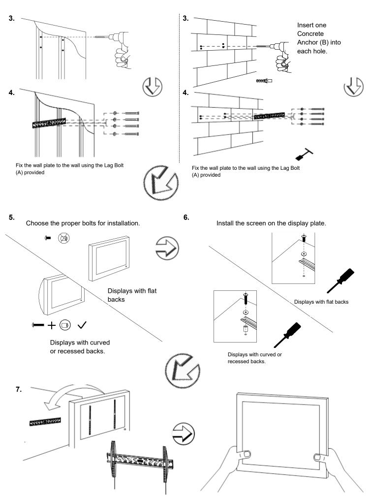
Place the display plate with the tv on the wall plate.
